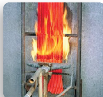
Fire Resistant Cable Testing
